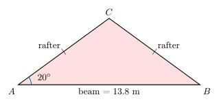
Students should write:  $\cos(20^\circ) = \frac{\text{half-beam}}{\text{rafter}} = \frac{6.9}{\text{rafter}}$ , then calculate:  $\text{rafter} = \frac{6.9}{\cos(20^\circ)} \approx 7.35 \text{ m.}$
